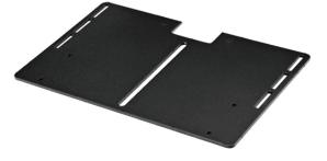
The **PM-CMP** was designed as an add-on for the standard cam tongue on PM series stands. When a set mounted codec is required, the **PM-CMP** features a large surface designed to fit most of today's codecs and wider cameras such as the \*EagleEye<sup>™</sup>. Slots for mounting straps and a long adjustable slot for a 1/4-20 bolt. Includes mounting hardware.
